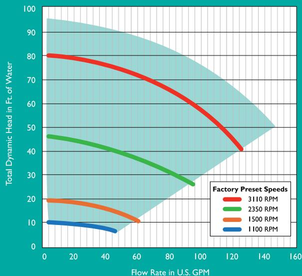
NOTE: The chart above demonstrates performance rates at factory preset speeds of 1100 RPM, 1500 RPM, 2350 RPM and 3110 RPM. However, flow rates can also be custom programmed between the ranges of 1100 RPM and 3450 RPM as indicated by the green tint.
