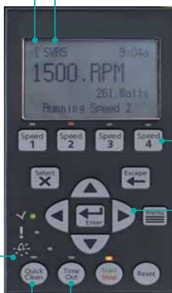
**Function buttons** to set speeds for separate operations—filtration cycles, spas, cleaners, water features and more
